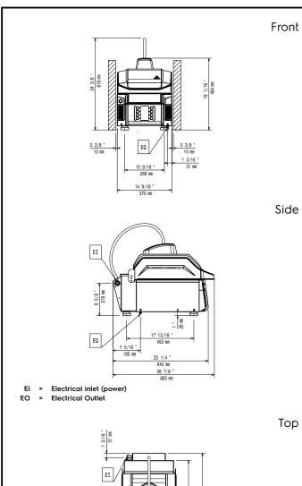
Supply voltage:220-230 V/1 ph/50 HzRated amps:12 ATotal Watts:2.7 kWPlug type:CE-SCHUKOInstallation:CerschukoClearance:190mm from rear vertical panel
